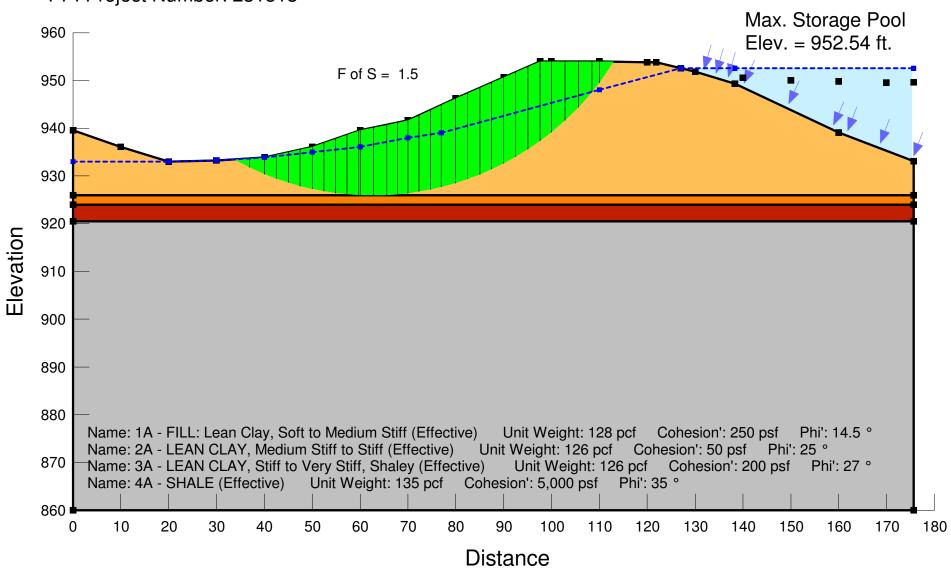
Periodic Safety Factor Assessment Asbury CCR Impoundment Static, Maximum Surcharge Pool Effective Stress Conditions Critical Cross Section PPI Project Number: 231518
