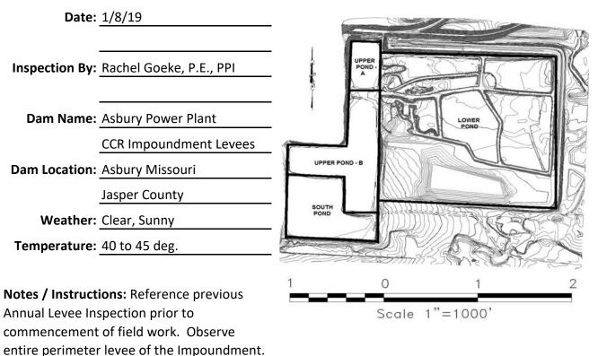
Summarize Overall Condition of Levee Embankments: <u>The overall condition of the perimeter</u> levee embankments is good. Evidence of sloughing or seepage was not observed during the inspection.
